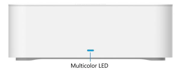
**LED** color Operation Meaning Solid Strong 5G connection (3 – 5 bars) **Blue** Blinking Weak 5G connection (1 – 2 bars) Solid Strong 4G connection (3 – 5 bars) Green Blinking Weak 4G connection (1 – 2 bars) White Blinking Factory reset  $\bigcirc$ Yellow Solid Software update is in progress Solid Router is booting up Red Blinking No service, SIM error, or locked SIM card
