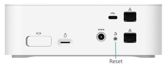
3. Press the recessed button for about five seconds until the device resets. The LED blinks white, then turns red. When it is green or blue, your FX3100 is ready.
